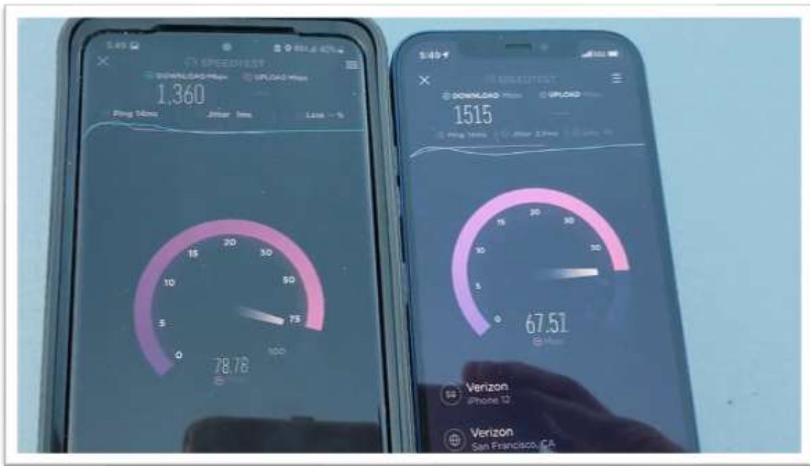
Figure 3 Two handsets combine for a total of 2.9 Gbps (downlink) and 145 Mbps (uplink)
